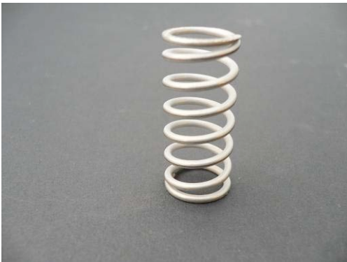
Pressure spring DF 2x12,6x32x5,5x1.4310 Art. No. 960066
